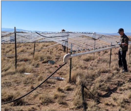
Left: plastic strips catch water and release it into a pipe which fills a reservoir container. Right: inverted plastic strips let water fall to the ground. Photos: Mariah Patton
