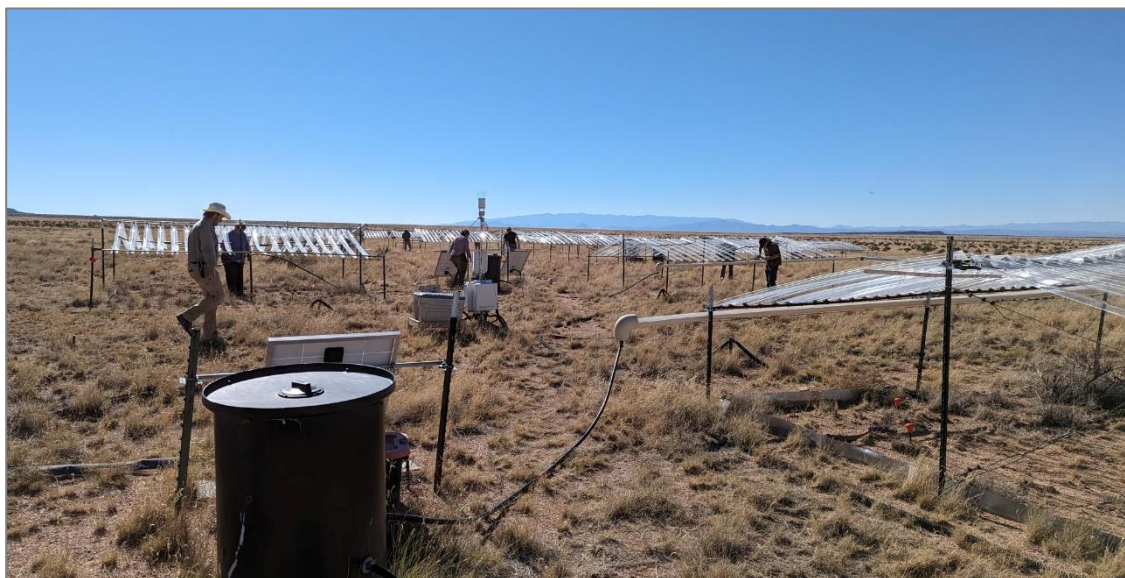
The black container stores water from one plot to be pumped to another plot. Solar panels provide power. Photo: Mariah Patton
